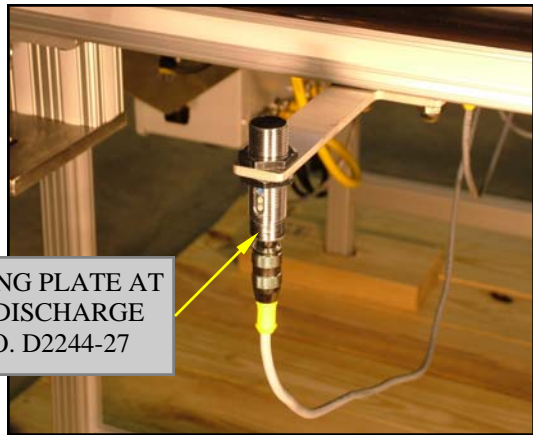
PE 3 SENSING PLATE FOR CLEAR TO LIFT PART NO. D2244-27
